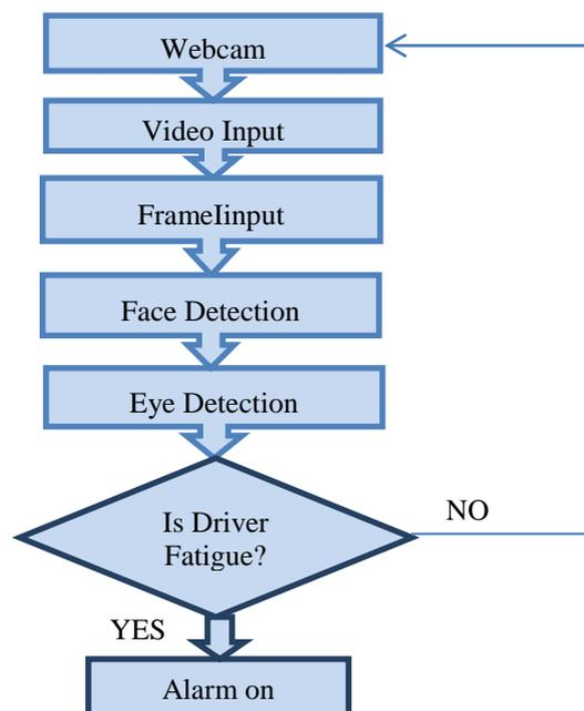
Figure 2: Flowchart of Driver Drowsiness Detection System
