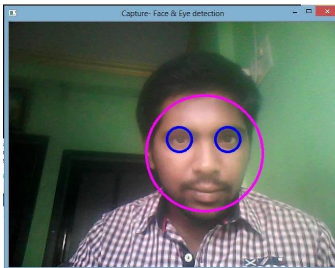
Figure6. Photography of face and eye detection
