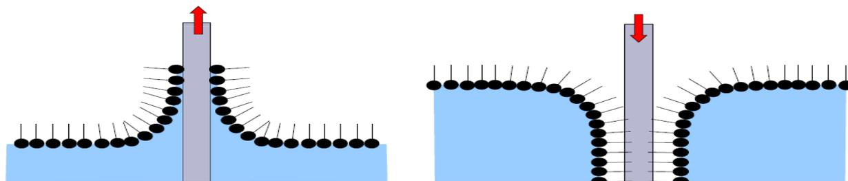
Figure 5. Schematic presentation of Langmuir-Blodget Technique for hydrophilic and hydrophobic substrates. (Zoran Jaksic 2010)
