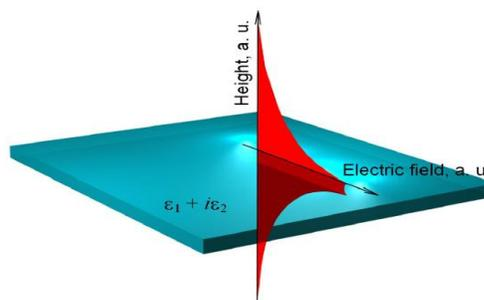
**Figure2.** Long-range surface-plasmon-polariton (SPP) propagation on a self-supported nanomembrane. "1"; "2: Dielectric functions. a.u.: Arbitrary units.( Zoran Jaksic 2011)
