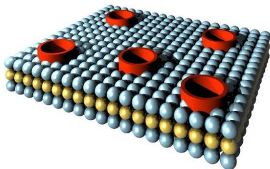
**Figure1.** Artificial ion channels (red cylinders) built into a three-layer nanomembrane.( Zoran Jaksic 2011)
