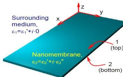
Figure 4. Basic configuration of a freestanding nanomembrane guide for long-range surface plasmon polariton propagation (metal-dielectric interface) (Kenichi Takahata, 2009)
