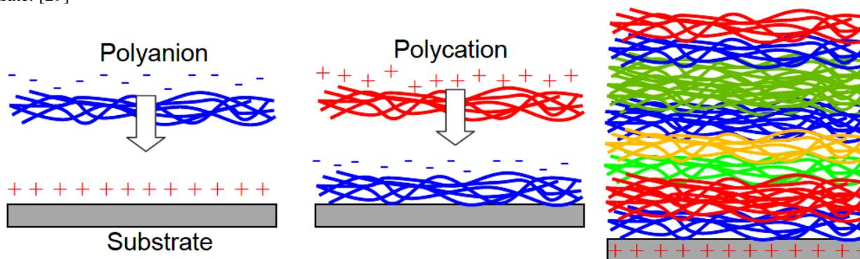
Figure 6. Layer-by-layer nanomembrane assembly technique. Left: assembly of the first layer; middle: assembly of the second layer; right: final structure (.Zoran Jaksic 2010)
