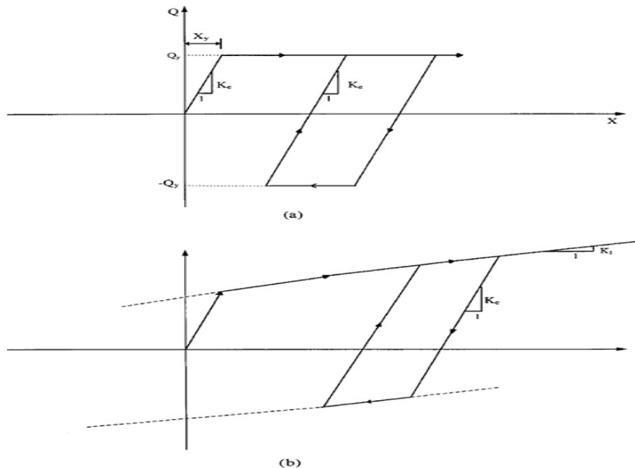
Fig 4: (a) Elastic-perfectly plastic model; (b) General bilinear model
