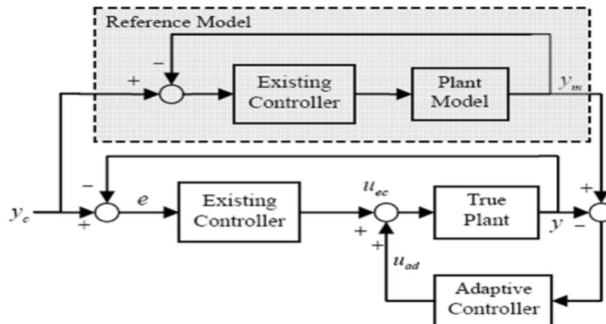
Fig 3: The closed loop reference model following adaptive augmenting architecture [19]
