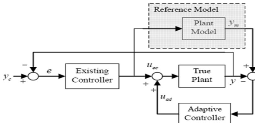
Fig 1: The open loop reference model following adaptive augmenting architecture [16]
