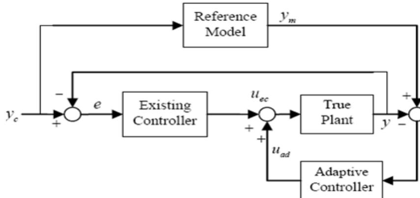
Fig 2: The arbitrary reference model following adaptive augmenting architecture [23]
