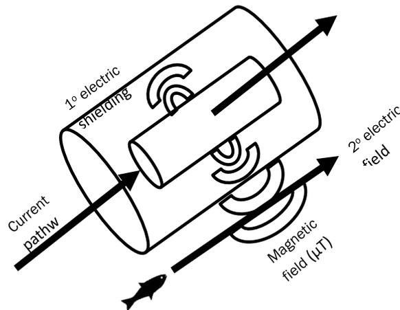
**Figure 2.** Representation of how an EMF is generated from a partially shielded subsea cable.
