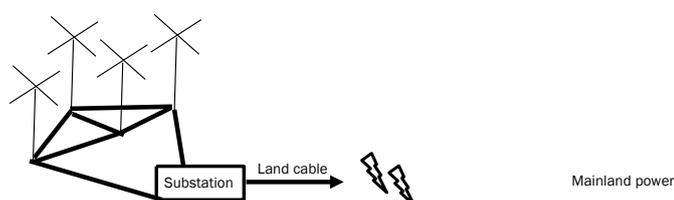
**Figure 1.** Representation of an offshore wind farm with a connecting network of subsea cables linking to an offshore substation before electricity is redirected through a cable to land.
