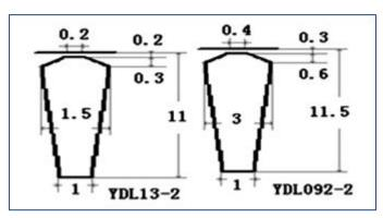
Fig. 3Rotor slots dimensions
