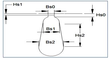
Fig. 4Slot dimension of rotor
