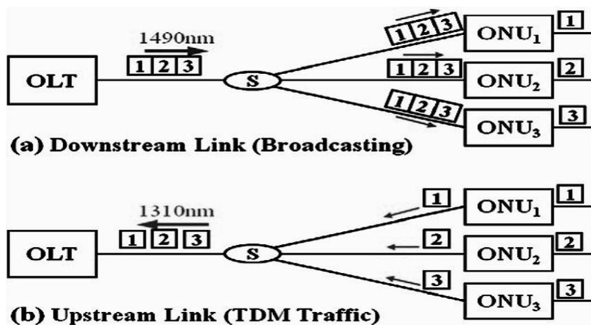
Fig.3. TDM-PON architecture
