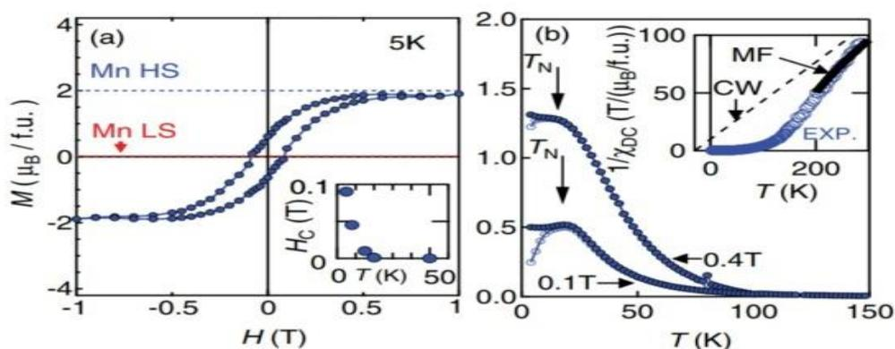
Magnetic properties shown in Figure 7 revealed FC and ZFC measurements. These observations propound that the temperature associated with the peak is of the order of anti-ferromagnetic temperature. Neel temperature calculated from the rise of FC and ZFC was reported at 21 K. Also reported that ground state of the material is ferromagnetic. This result is confirmed by magnetic measurements of the material with  $\text{Mn}^{+3}$  at high spin state.
