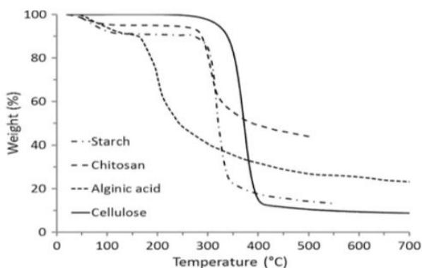
Figure 2. Thermogravimetric curves of selected carbohydrate flame retardants [11].
