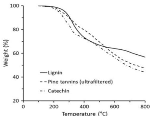
Figure 3. Thermogravimetric curves of selected Phenolic Flame retardant compounds [8,17].
