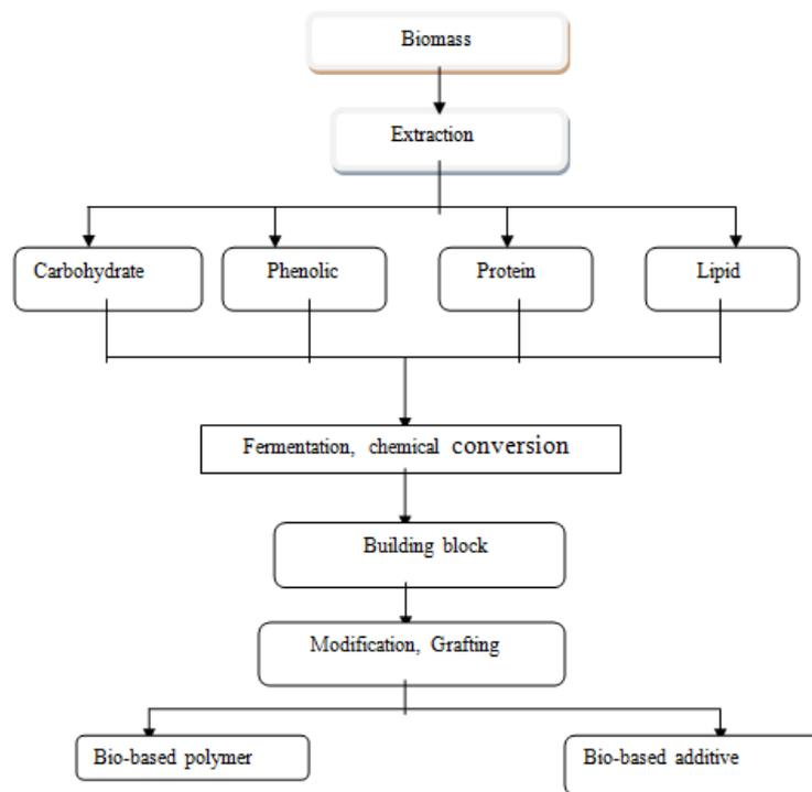
Figure 1. The process of obtaining bio-based additives for polymer [4].
