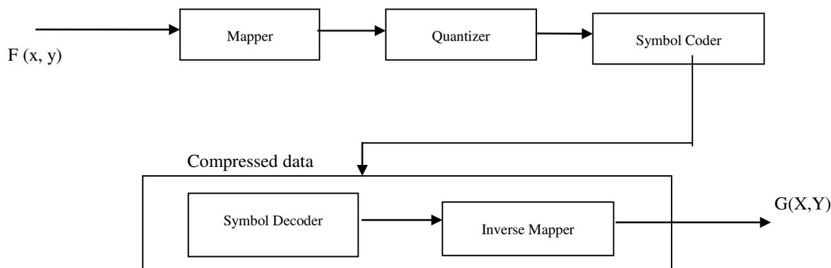
Figure 1: Functional Block Diagram of an Image Compression System
