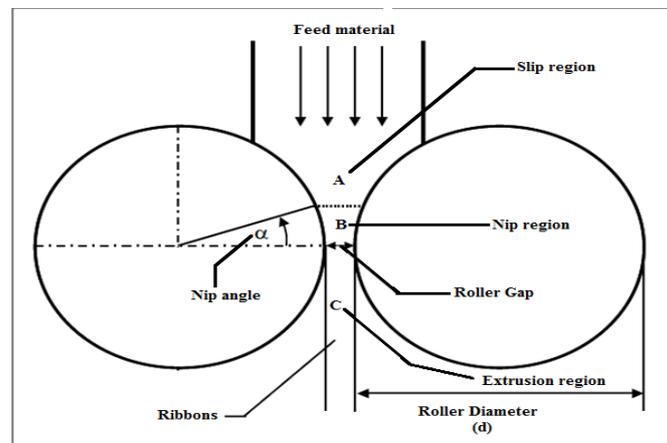
Figure No: 1 Process of roller compaction
