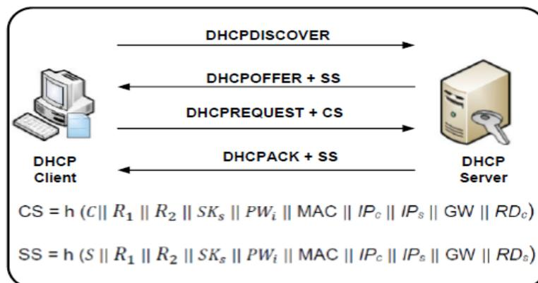
Figure 3: the DHCP message exchange using MA technique
