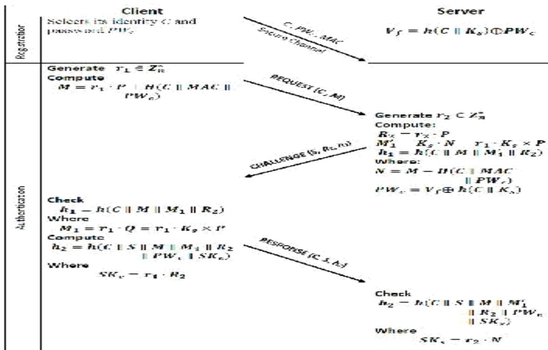
**Figure 2:** Flow diagram for EAKM technique
