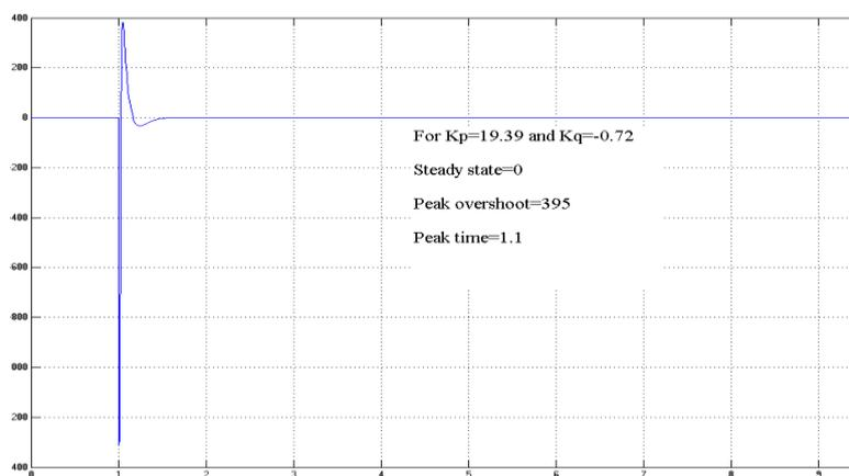
Fig. 4(c): Fin deflection rate for  $K_p = 19.39$  and  $K_q = -0.72$
