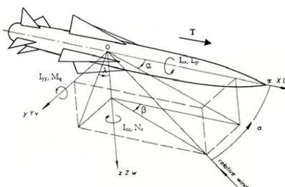
Fig.1: Missile Autopilot with Motion variable notations
