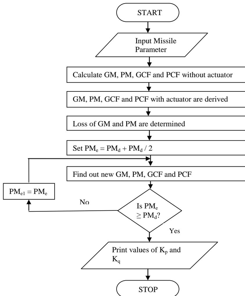
Fig. 3: Flow chart for Control Gain design
