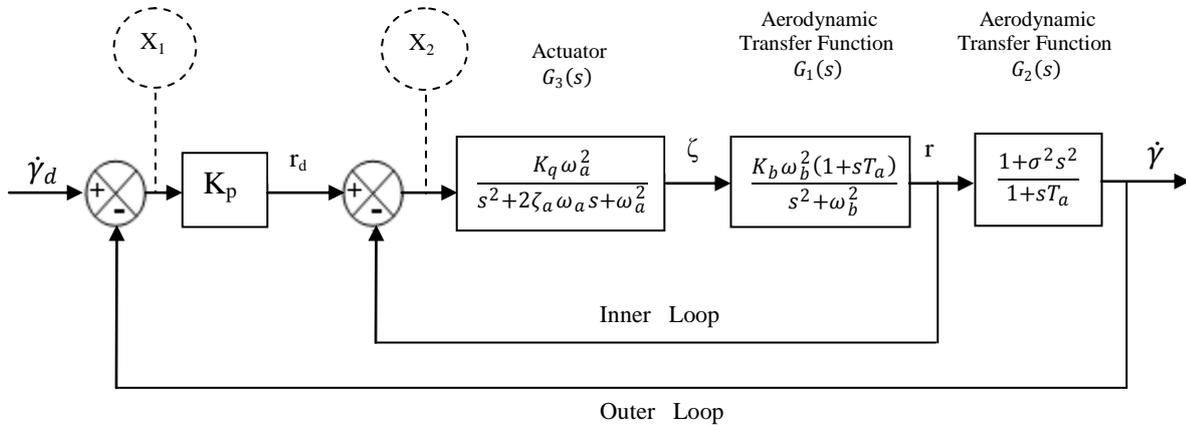
Fig.2: Flight Path Rate Demand Autopilot in Yaw Plane
