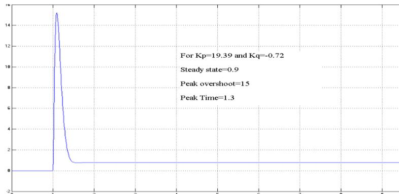
Fig. 4(a): Body rate for  $K_p = 19.39$  and  $K_q = -0.72$
