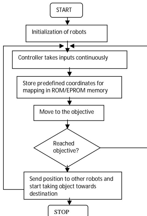
Fig.3 Flow Chart of Overview of Algorithm
