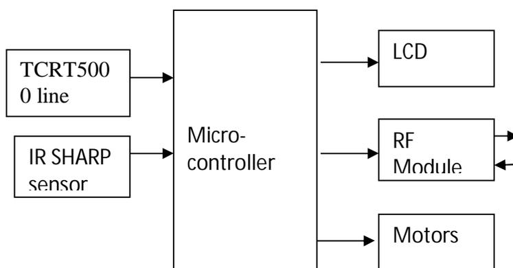
Fig.1Block Diagram of Robot
