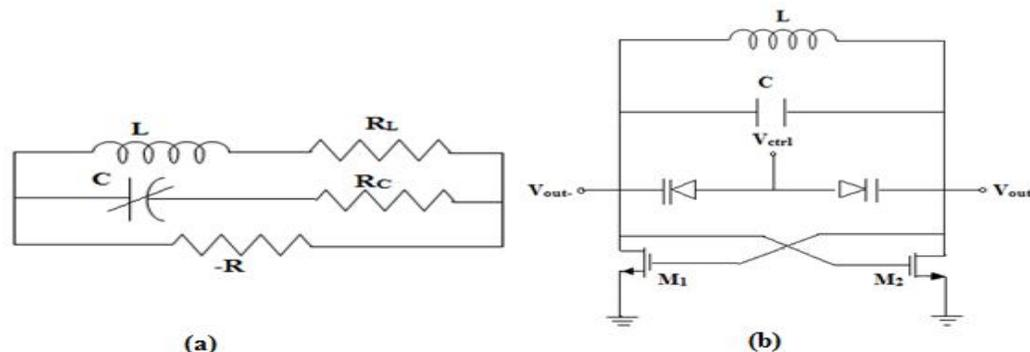
Fig. 1 (a) Basic LC VCO (b) Cross Coupled Oscillator
