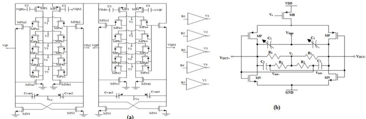
Fig. 8 (a) Active VCO (b) Fully differentially BPF based oscillator.
