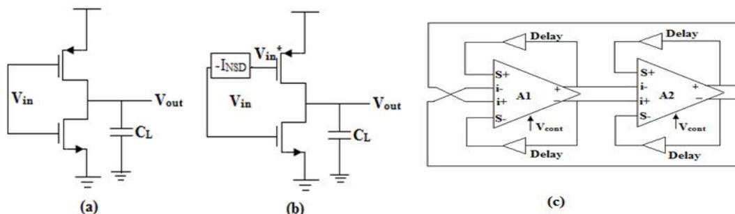
Fig. 7 (a) Conventional Delay cell (b) NSD cell (c) Block diagram of modified 2 stage ring oscillator.
