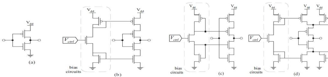
Fig 5: Inverter (a) basic type (b) current starved with output switching (c) current starved with power switching (d) current starved with symmetrical load.
