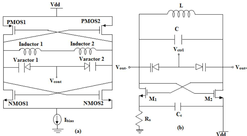
Fig. 2 (a) Cross Coupled Oscillator (b) Complimentary Cross Coupled Oscillator
