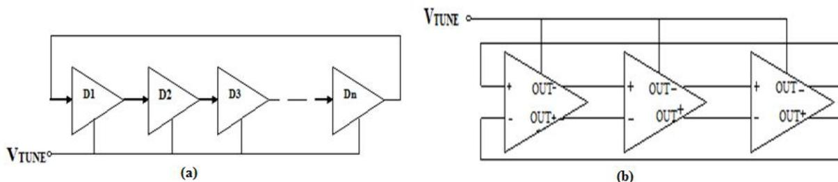
Fig. 4 (a) Single Ended Ring VCO (b) Differential loop Ring VCO
