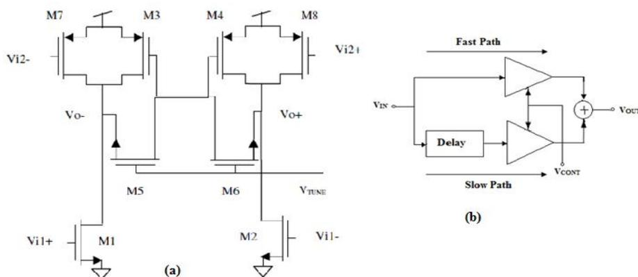
Fig 6 (a) Conventional Differential delay cell (b) Implementation of each 3 stage delay
