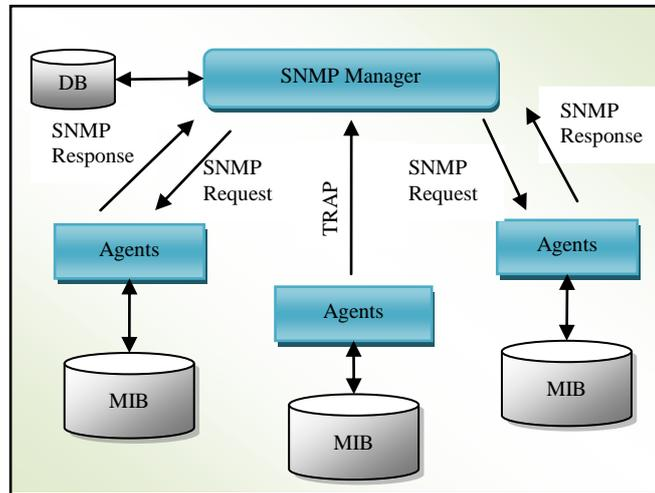
Fig 1. Centralized NMS architecture
