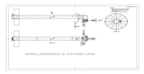
The atomising nozzle assembly consists of Spray Plate (Atomiser), which is secured to the nozzle body by means of a cap nut. The atomising agent (Compressed air / Steam) enters the oil gun through the lower part of the stationary union and the oil enters the upper part. They are carried separately through the entire length of the gun by means of two parallel oil gun pipes.
