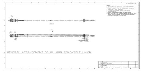
Guides on the outer oil gun pipe maintain the concentric position of the oil gun with respect to stationary part. The flexible tubing adapts the gun to vertical tilting of the wind box nozzle and serves to absorb the differences in expansion between the pipes.
