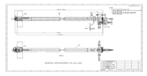
The stationary union is welded to a tube called connecting tube. The stationary union provides connection for admission of oil and atomising agent and at the same time couples the removable part. The gun engagement limit switch is actuated by the actuator lever when the oil gun removable part is engaged onto the stationary part and coupled. The limit switch contacts serve to indicate the control system that the oil gun is engaged in position and is ready for firing.
