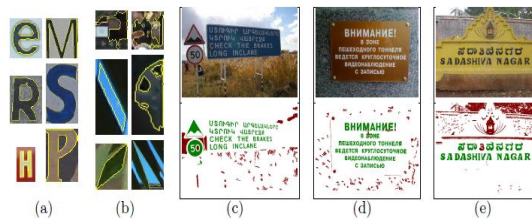
Figure 2:Character/non-character MSER classifier: (a) Character and (b) non-character training samples (MSER boundaries marked yellow). Initial MSER classification for (c) Armenian, (d) Russian and (e) Kannada script (character regions marked green, Non character regions marked red). Note: The training set contains only 1227 character samples of Latin script and 1396 non-character samples
