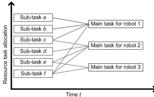
Fig 6 Task execution example using parallel model in task the executor
