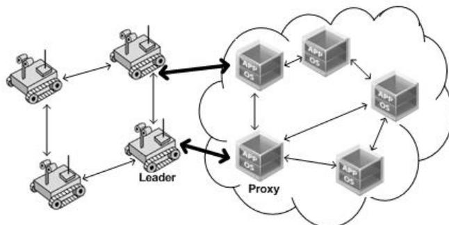
Fig.2 Proxy-Based cloud robotics model[3]
