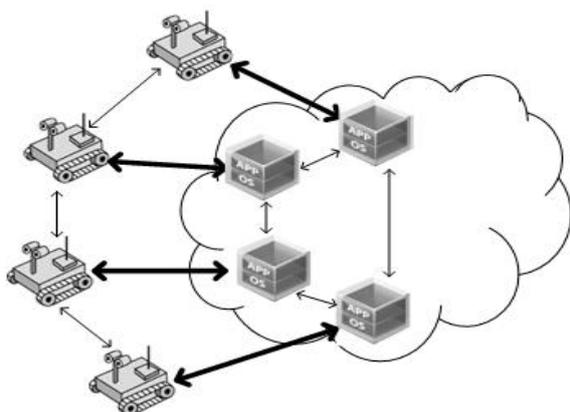
Fig.4 Clone-Based cloud robotics model[3]
