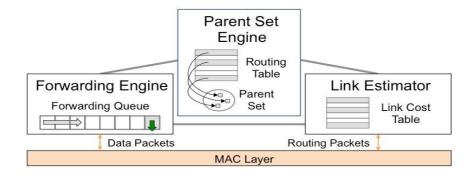
Fig.1. Main components of CTP+PPS.
