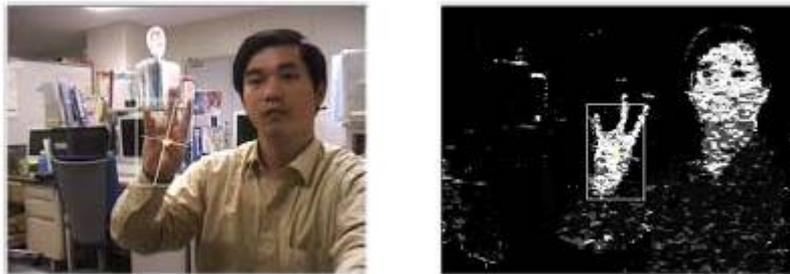
Fig.2. Orientation of the flesh probability distribution marked on the source video image from CCD camera.
