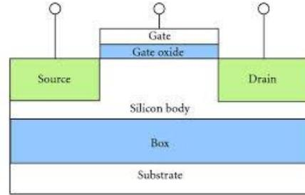
Figure 1: SOI MOSFET Structure
