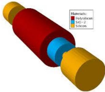
Figure 6: GAA MOSFET Structure
