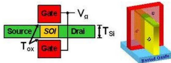
Figure 2: Symmetric common DG-MOSFET Structure
