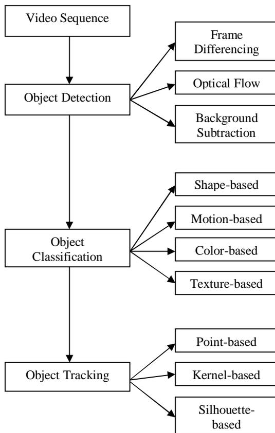
Fig 1: Basic steps for tracking an object [8]
