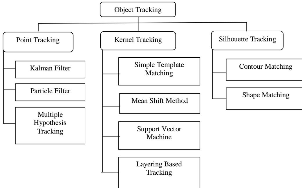
Fig 2: Types of Object Tracking Methods [10]
