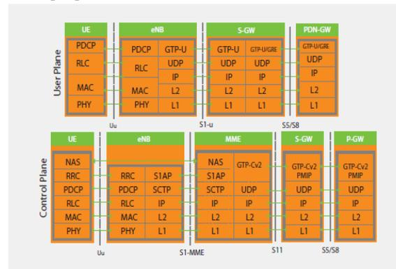
Figure 6: LTE User-Plane and Control-Plane Protocol Stacks
