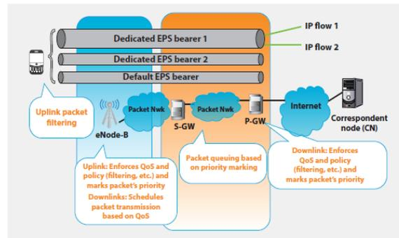
Figure 5: QoS Assignment on EPS Bearers
