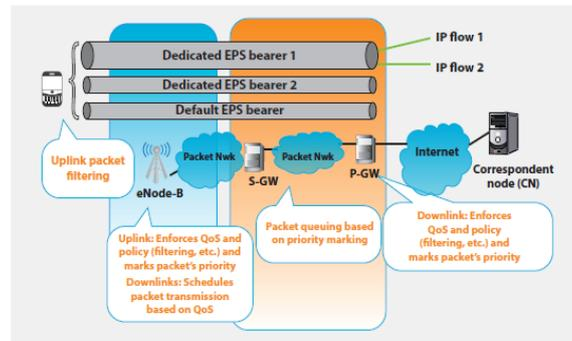
Figure 5: QoS Assignment on EPS Bearers
