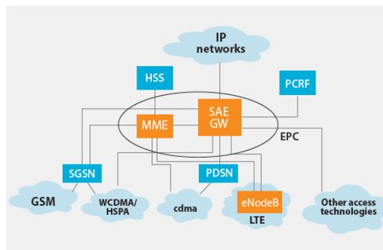
**Figure 3: Simplified View of LTE Network Architecture**
