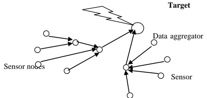
Fig. 2 - Data aggregation in Wireless Sensor Network
