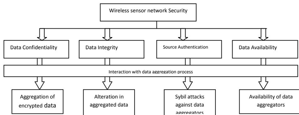
Fig. 3 - Interaction between data aggregation process and security requirement
