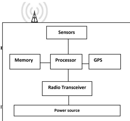
Fig. 1 - Components of WSN Node
