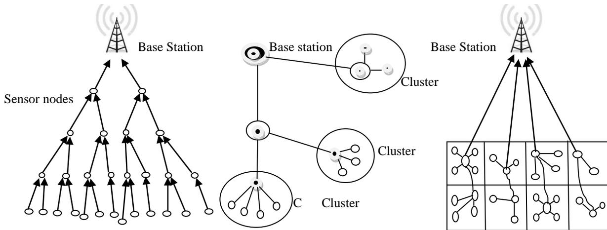
Fig 4. Tree based, Cluster based and Chain based Data Aggregation in Wireless sensor networks
