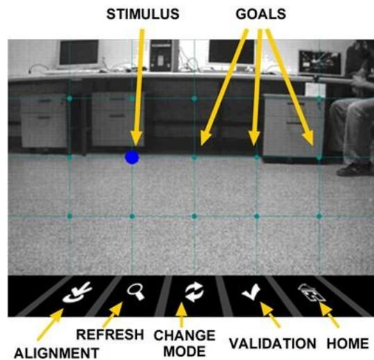
Fig. 3. Visual display in robot navigation mode (upper section of figure) and in camera exploration mode (lower section of figure). An individual visual stimulus represented by a blue circle is shown in both figures; however, the real stimulation process was accomplished by means of rows and columns.
