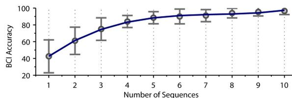
Fig. 4. BCI classification accuracy versus the number of sequences of the stimulation process. Mean and standard deviation values are shown for all the participants in the calibration trials of the *Evaluation of Brain-Actuated Telepresence* (see methodology). Ten fold cross-validation was applied.
