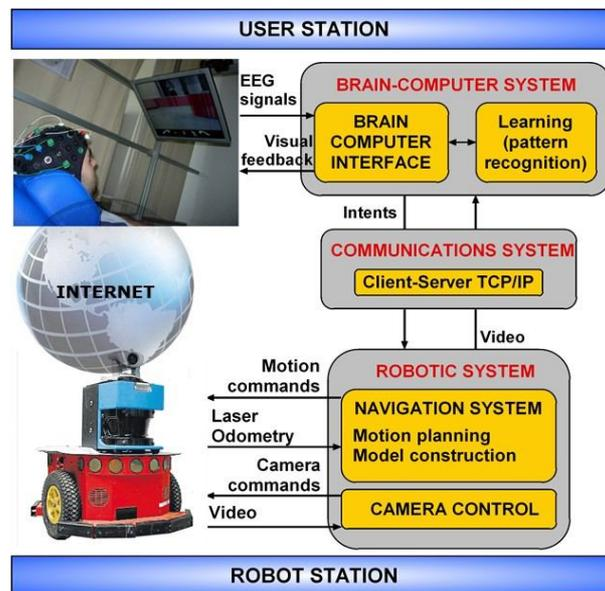
Fig. 1. Design of the robotic telepresence system actuated by a non-invasive brain-computer interface with main modules and information flow.
