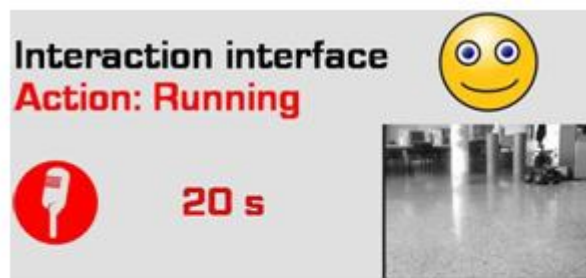
Fig. 3. Robot station graphical interface, displayed in the laptop placed on the robot. This interface shows the actions that the user is performing, his emotional state, and whether video and audio is being sent to the user. Furthermore, when the robotic device is sending video and audio, it displays that video and the resting time to stop the transfer.
