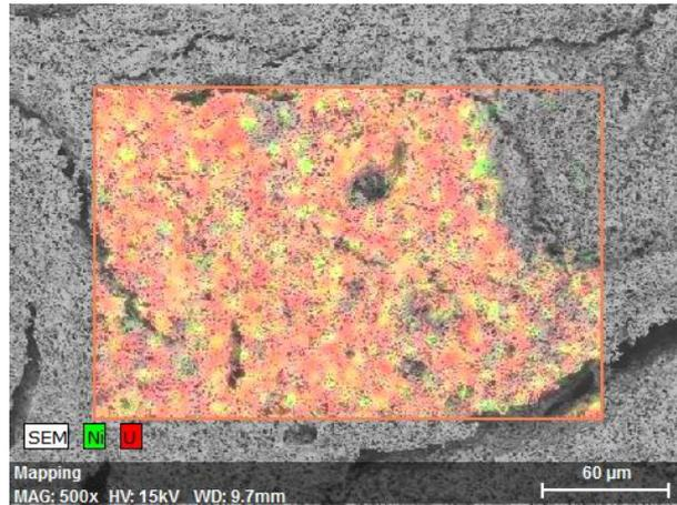
**Figure 4.** SEM/EDS mapping of the distribution of U and Ni within the air dried sphere.
