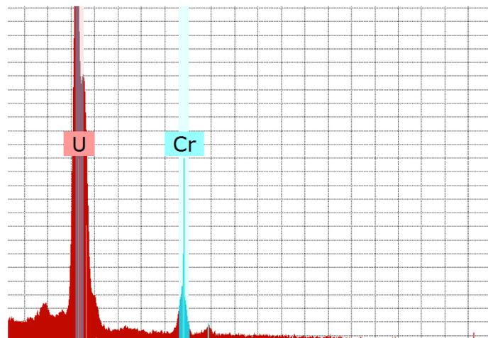
**Figure 9.** The EDS spectrum of inside the sphere of a U/Cr sample after carbothermal reduction.
