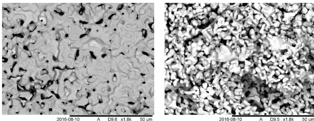
**Figure 15.** A SEM image of the top (left) and bottom (right) surface of the U/Cr pellet after sintering in argon.
