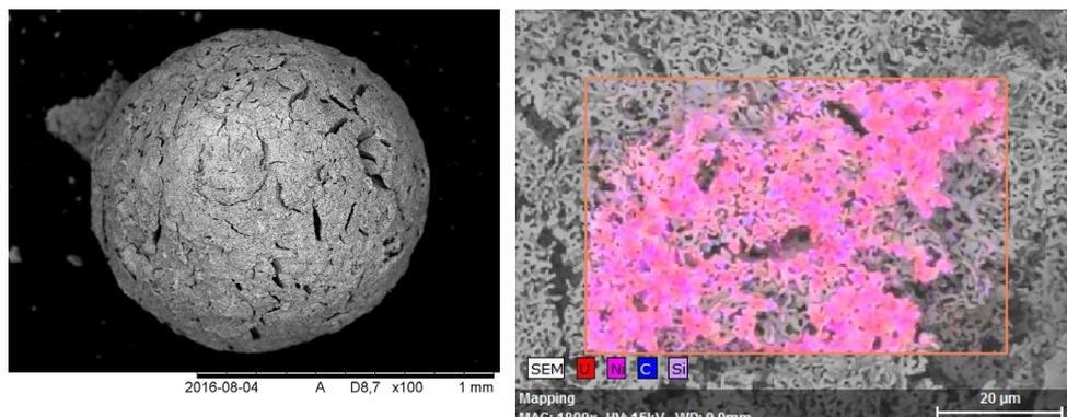
**Figure 11.** SEM image of a sphere containing uranium and nickel after nitridation (left). SEM/EDS mapping of the distribution of U and Ni inside a nitrided sphere (right).
