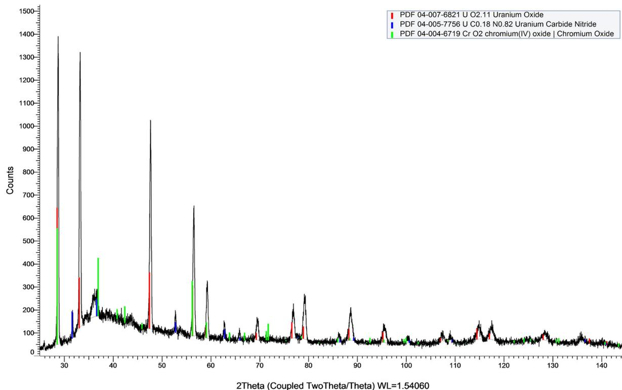
**Figure 19.** XRD pattern of the U/Cr pellet after sintering in Argon. Three phases corresponding to  $\text{UO}_2$ ,  $\text{CrO}_2$  and UN were detected on the surface.
