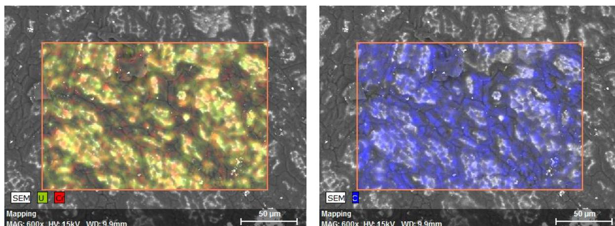
**Figure 3.** The SEM/EDS mapping of uranium and chromium (left) and carbon (right) distribution on the surface of an air dried sphere prepared from uranium and chromium nitrate.
