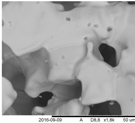
**Figure 25.** SEM image of the top surface of the U/Al pellet after sintering in argon.
