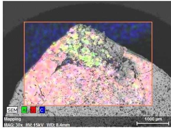
**Figure 24.** SEM image of the U/Ni pellet bottom showing the segregation of nickel from uranium along the grain boundaries.
