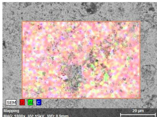
**Figure 13.** SEM/EDS mapping of a sphere containing uranium and aluminum after nitridation.
