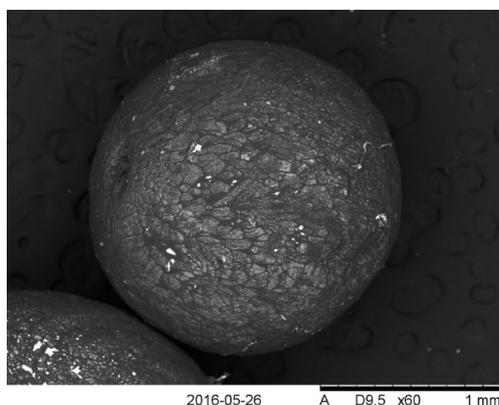
**Figure 2.** The SEM image of a single air dried sphere prepared from uranium and chromium nitrate.
