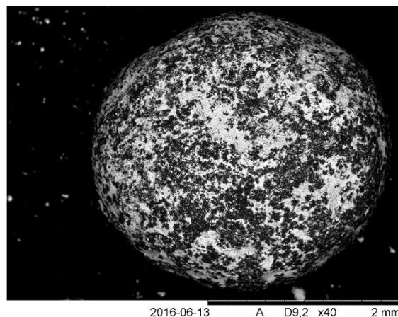
**Figure 5.** The SEM image of a single air dried sphere prepared from uranium and aluminum nitrate.
