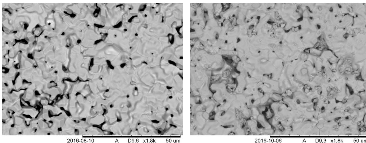
**Figure 27.** SEM image of a chromium doped pellet surface before (left) and after (right) the dissolution test.
