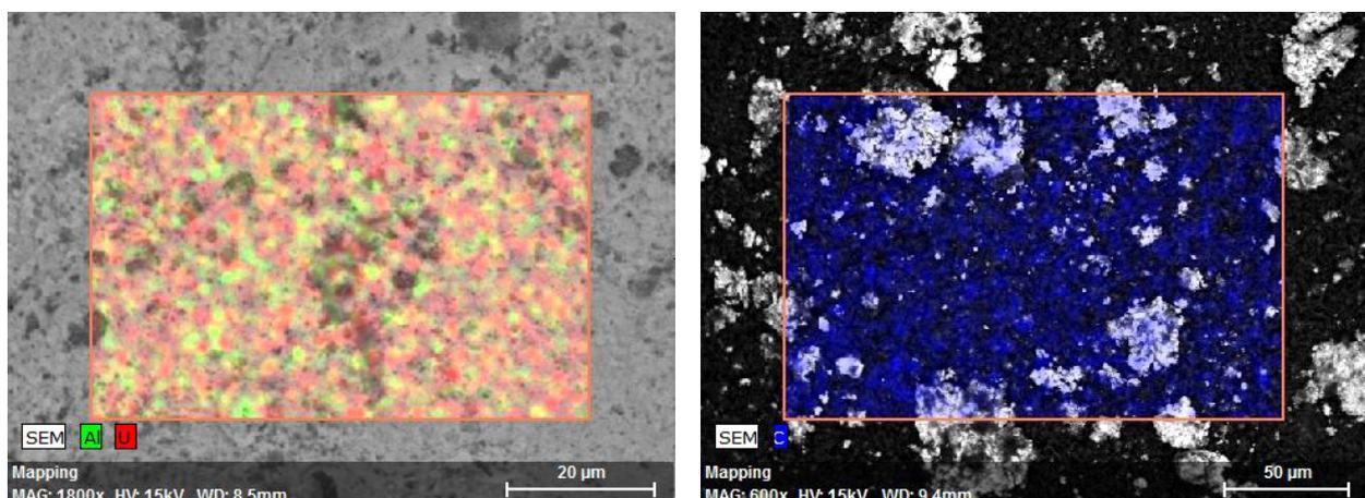
**Figure 6.** SEM/EDS mapping of uranium and aluminum (left) and carbon (right) distribution on the surface of an air dried sphere prepared from uranium and aluminum nitrate.
