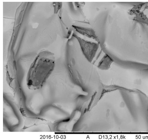
**Figure 22.** SEM image of the bottom surface of the U/Ni pellet after sintering in argon. The dark grey spots possibly consist of  $UNi_5$ .
