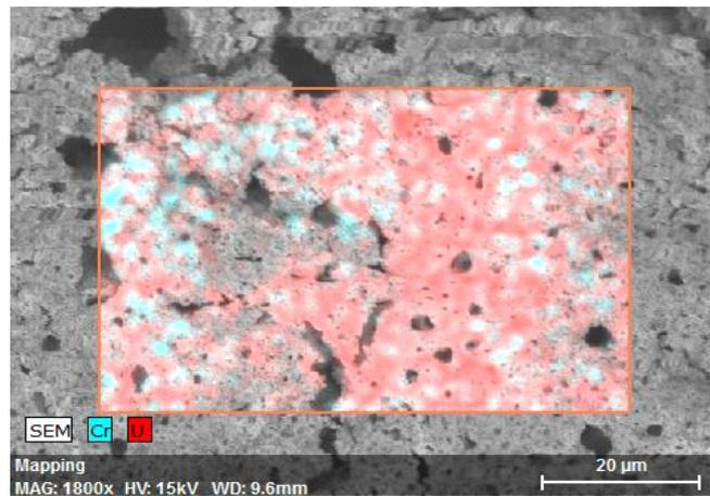
**Figure 8.** SEM/EDS mapping of the distribution of U and Cr inside a nitrated sphere.
