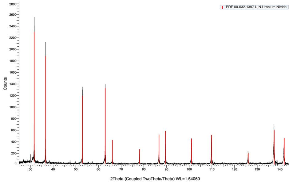
**Figure 12.** XRD pattern of U/Ni sample after carbothermal reduction; the phase corresponds to UN.
