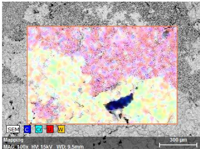
**Figure 17.** A SEM image of the U/Cr pellet bottom showing an interaction with tungsten from the tungsten plate.
