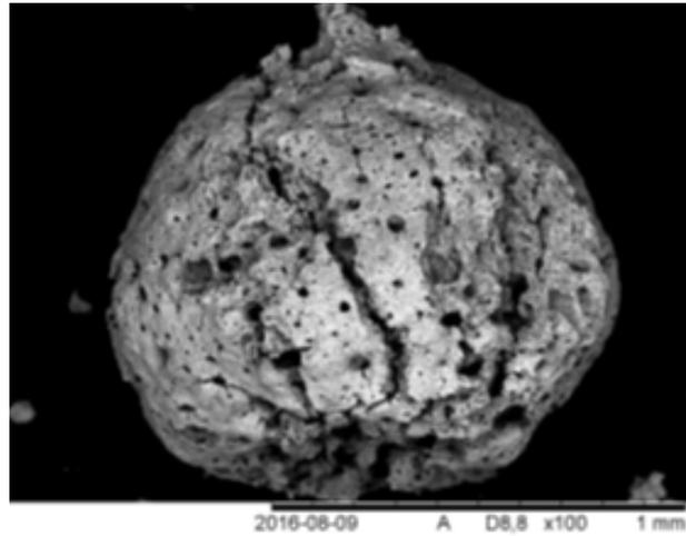
**Figure 7.** SEM image of a sphere containing uranium and chromium after nitridation.
