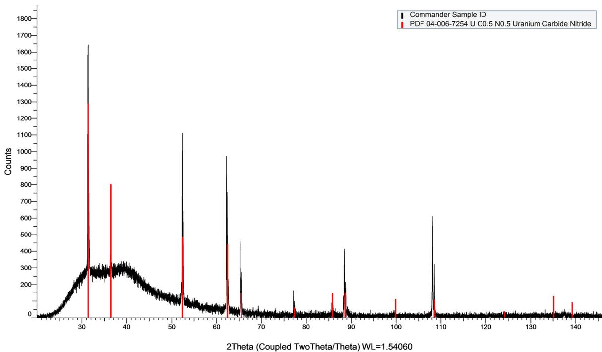
**Figure 26.** XRD pattern of the U/Al pellet surface after sintering in argon.
