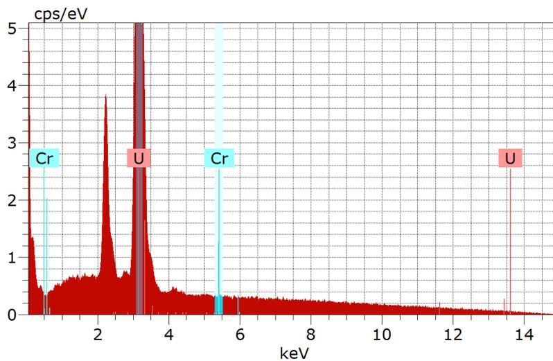
**Figure 18.** The EDS spectrum of the top of the U/Cr pellet after sintering in argon, showing a nearly complete absence of chromium on the surface and an unidentified peak.
