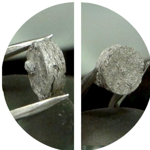
**Figure 23.** A photo of the U/Ni pellet after sintering in argon. Top surface on the left half, bottom surface on the right half.
