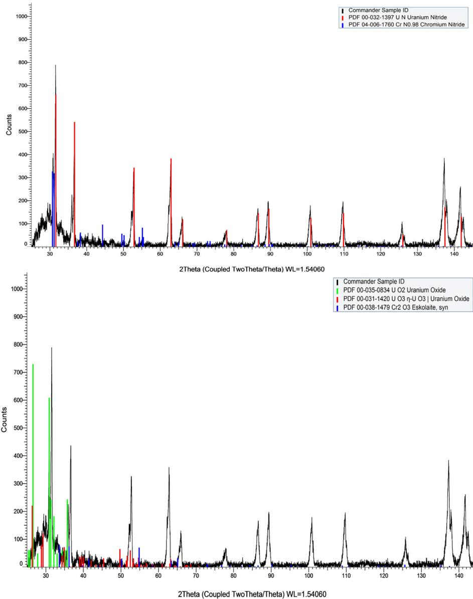
**Figure 10.** The XRD patterns of a U/Cr sample after carbothermal reduction. The major phase corresponds to nitrides (top), the second phase corresponds to oxides (bottom).
