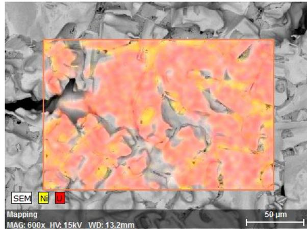
**Figure 21.** SEM image of the U/Ni pellet bottom showing the segregation of nickel from uranium along the grain boundaries.
