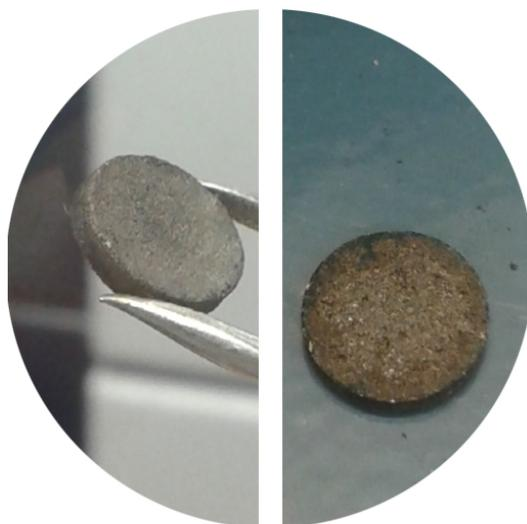
**Figure 20.** A photo of the U/Ni pellet after sintering in argon. Top surface is shown on the left half and the bottom surface on the right half.
