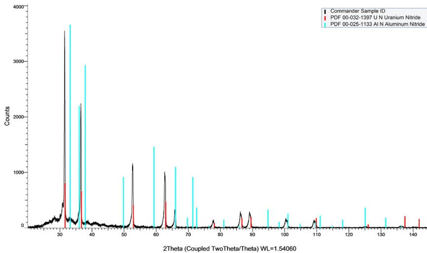
**Figure 14.** Consists of two XRD patterns which overlap each other patterns of U/Al sample after carbothermal reduction; the phases correspond to uranium nitride and Aluminum (III) oxide and aluminum (III) nitride.
