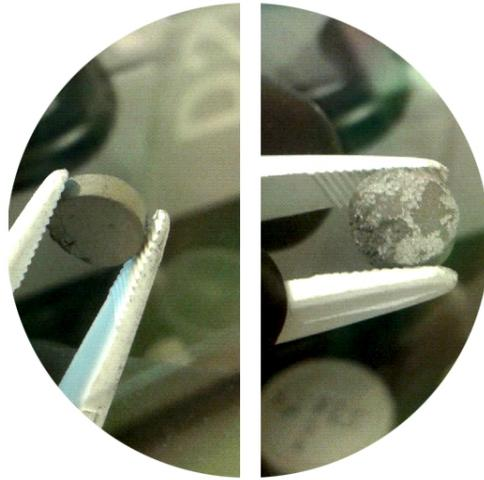
**Figure 16.** A photo of U/Cr pellet after sintering in argon. From left to right the top surface and the bottom surface.
