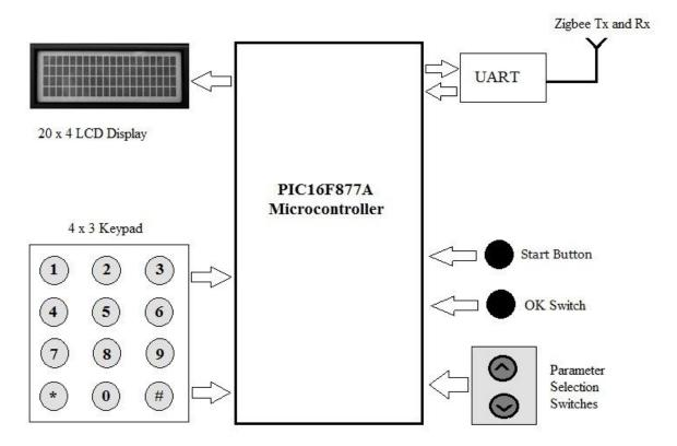
Fig. 2: The block architecture of the monitoring and Control node (The ADV user node).
