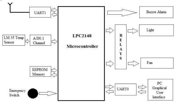
Fig. 1: The block architecture of the node to be monitored and controlled (The DISADV user node).
