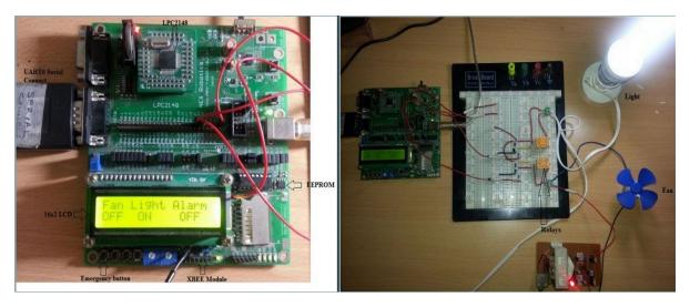
Figure 5: The DISADV user station composed of LPC2148 and associated peripherals.
