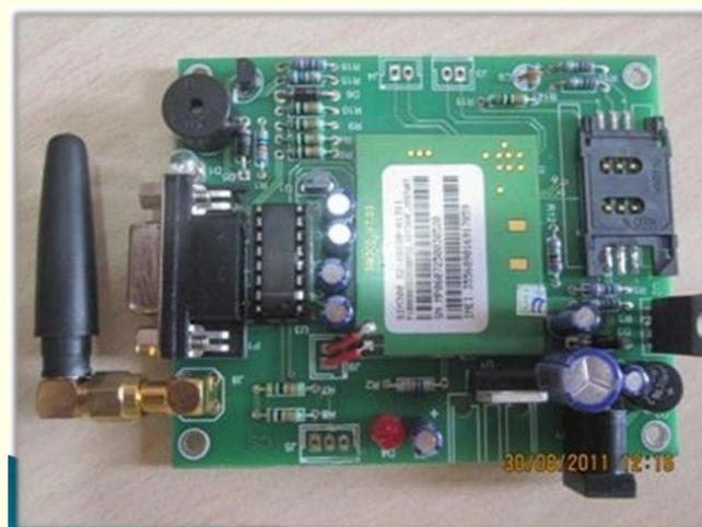
Fig 2 GSM Module
