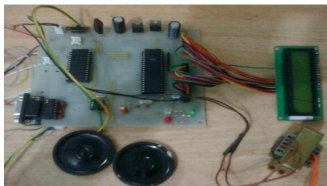
Fig. 6. ANC using microcontroller and ADC & DAC circuits
