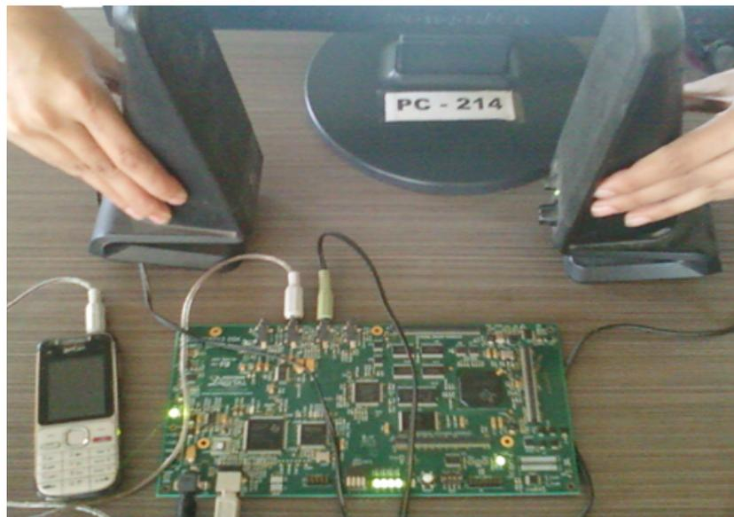
Fig. 7. ANC using DSP TMS320C6713
