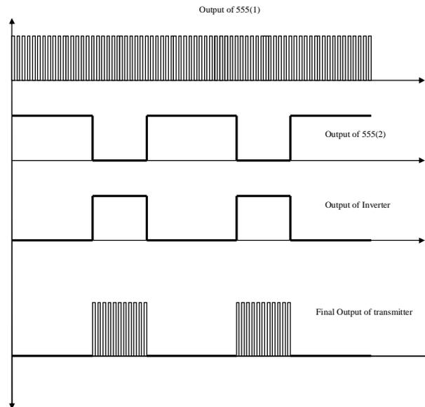
Fig.7. Hardware testing Results of Ultrasonic Circuit
