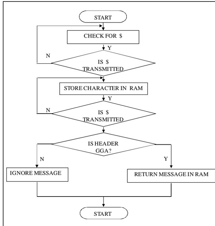
Fig.5. Flow chart for identification of GPS string
