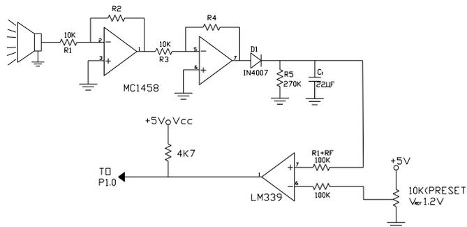
Fig. 2. Ultrasonic Receiver Circuit
