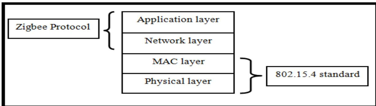
Fig.1 Protocol stack of Zigbee
