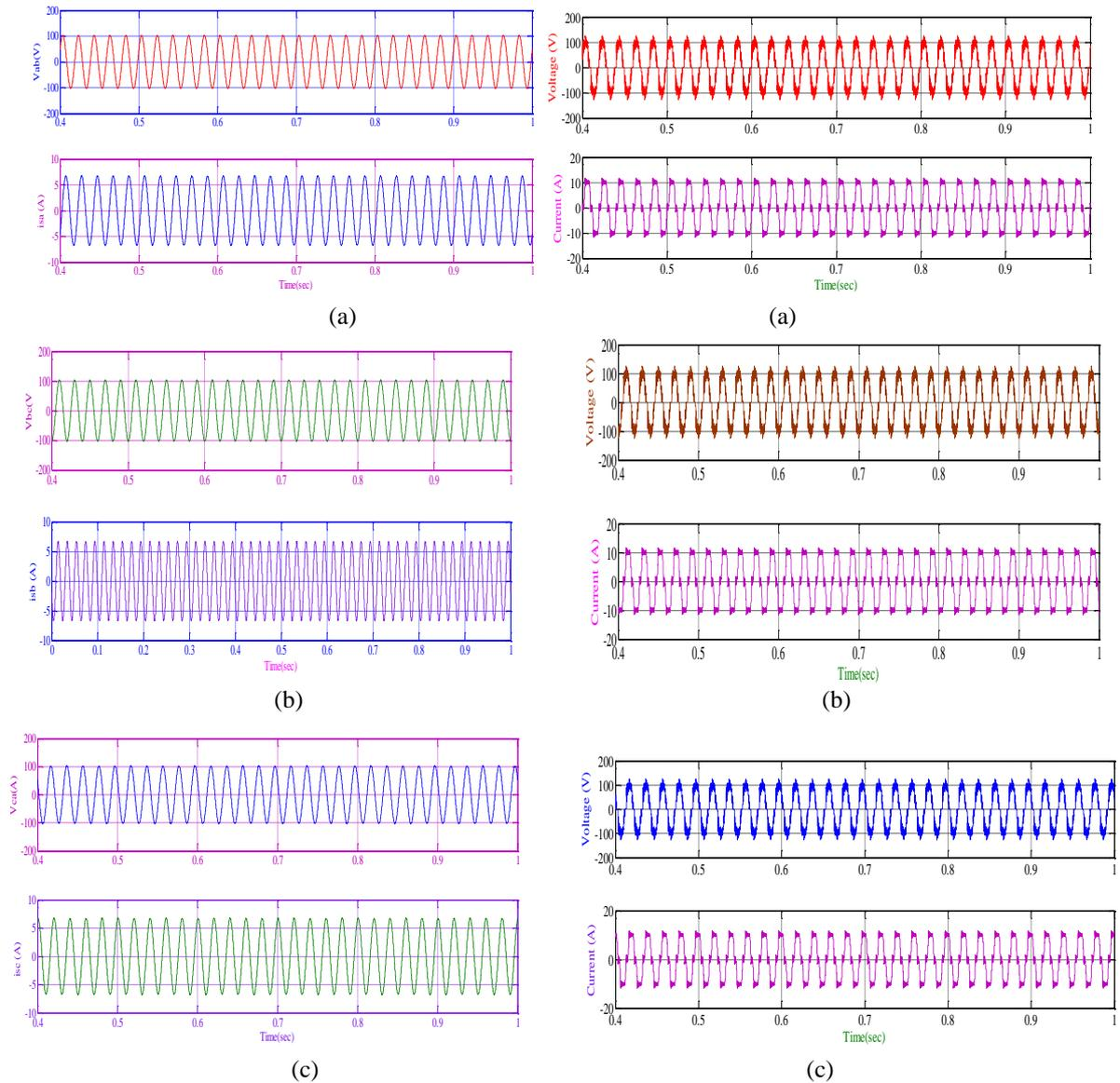
**Figure 7:** Steady-state performance of DSTATCOM at linear lagging PF load in ZVR mode.
