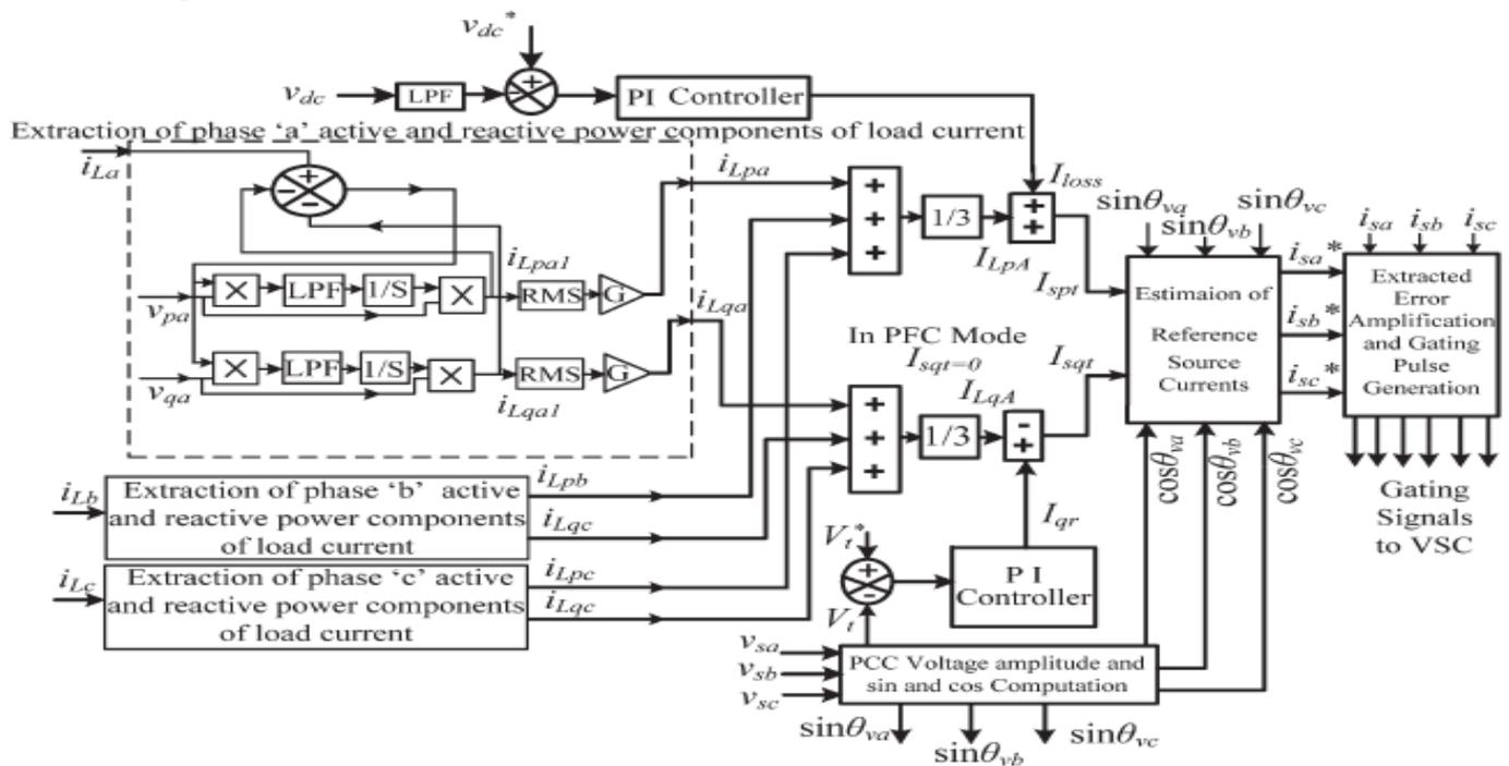
**Figure 1:** Generation of reference supply currents using Adaptive Filter.
