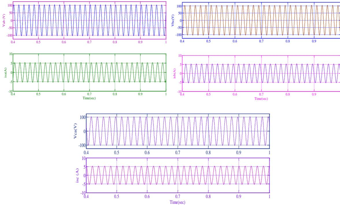
**Figure 4:** Steady-state performance of DSTATCOM at linear lagging PF load in PFC mode.
