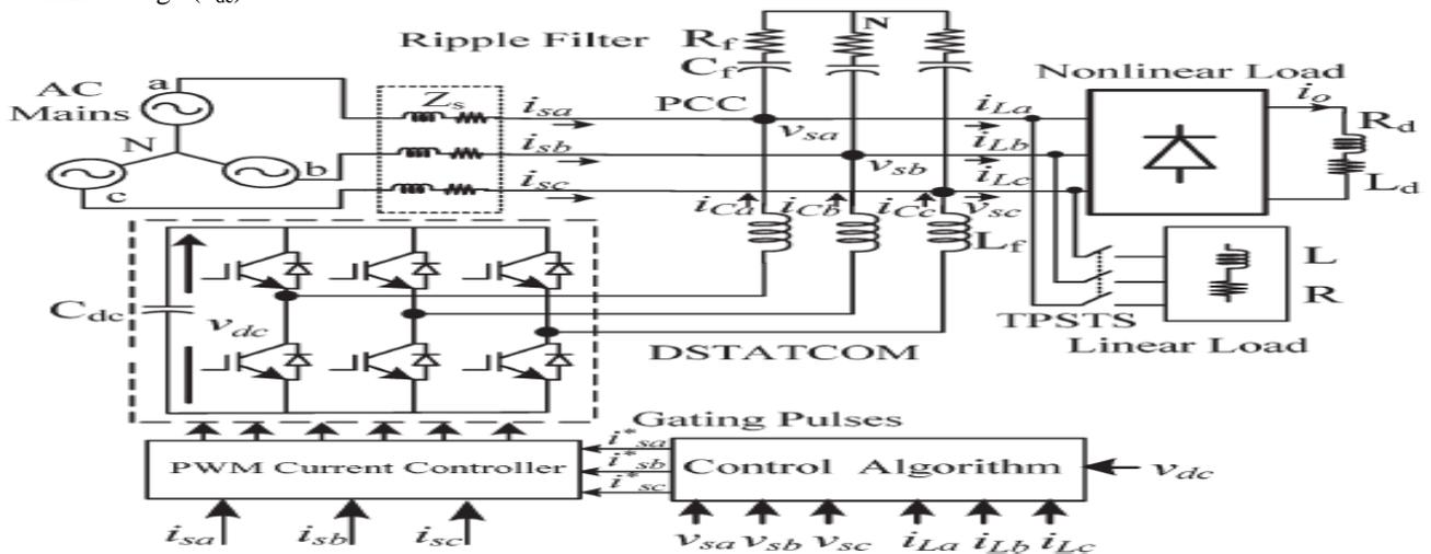
Interfacing inductors ( $L_f$ ) are connected at the ac side of the voltage source converter (VSC) for reducing ripple in compensating currents. The series-connected capacitor ( $C_f$ ) and resistor ( $R_f$ ) form the passive ripple filter installed at PCC in parallel with the load, and it is used for filtering the high-frequency switching noise of PCC voltages.
