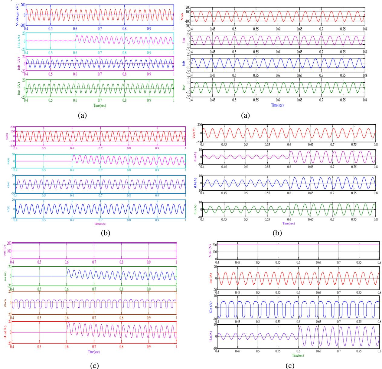
**Figure 6:** Dynamic performance of DSTATCOM at unbalanced linear loads
