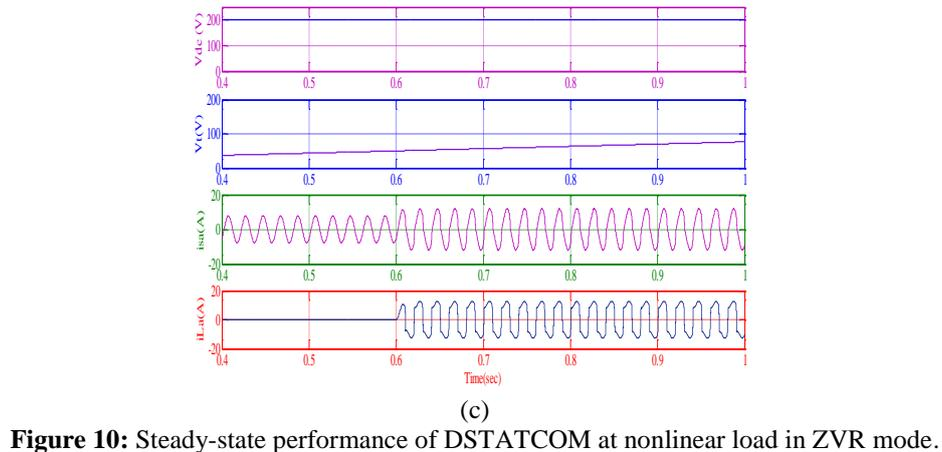
**Figure 10:** Steady-state performance of DSTATCOM at nonlinear load in ZVR mode.
