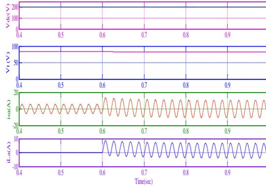
**Figure 9:** Variation of  $V_t$ ,  $i_{sa}$ , and  $i_{La}$  with  $v_{dc}$  under unbalanced linear loads.
