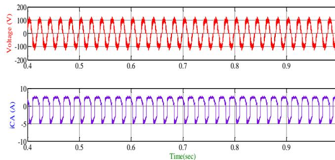
**Figure 8:** Steady-state performance of DSTATCOM at nonlinear load in ZVR mode.
