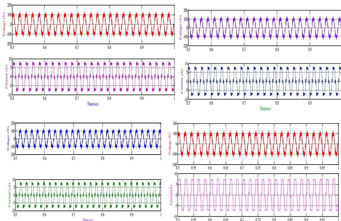
**Figure 5:** Steady-state performance of DSTATCOM at nonlinear loads in PFC mode.
