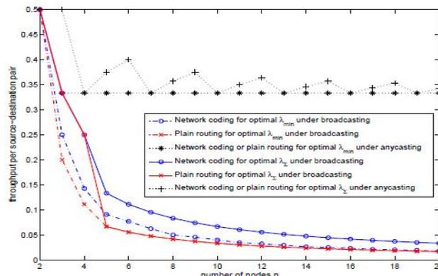
**Fig.4 Achievable throughput rates per source-destination pair under broadcast and ancast communication**
