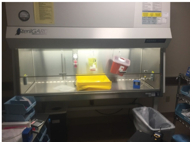
Figure 2. Typical air sampling set-up during a spill condition
