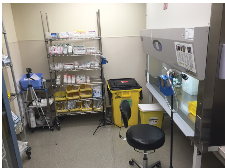
Figure 1. Typical air sampling set-up during a spill condition
