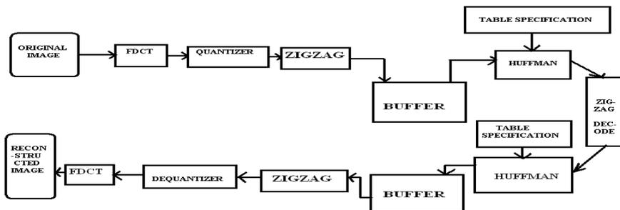
Fig.1.Block diagram of JPEG
