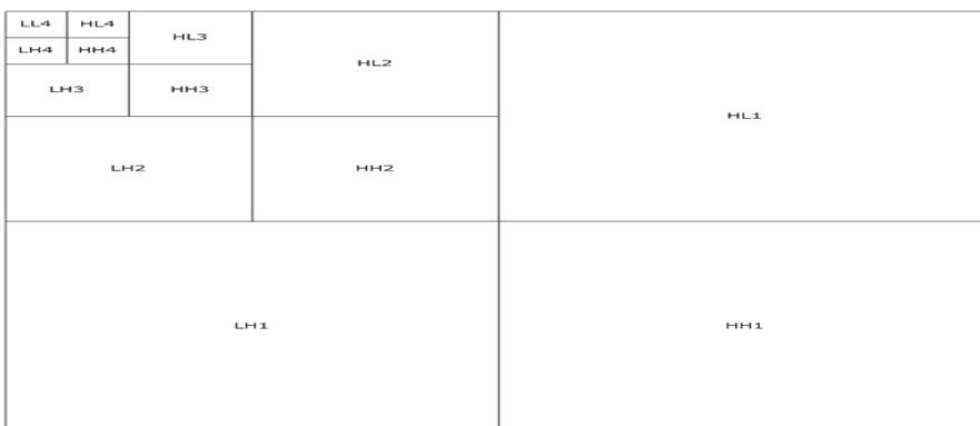
Fig.2.Four-level DWT decomposition of image tile
