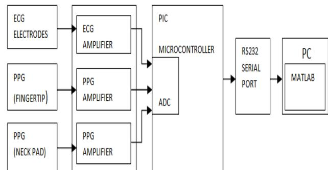
**Fig.2** Block Diagram of Ambulatory Device to Predict Myocardial Infarction and Ischemic Stroke
