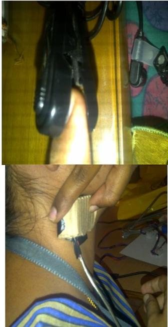
**Fig.6** Transmittance PPG sensor
