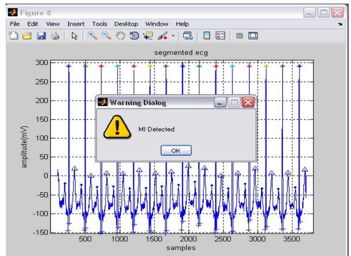
**Fig.9** Myocardial infarction detection through processed ECG signal
