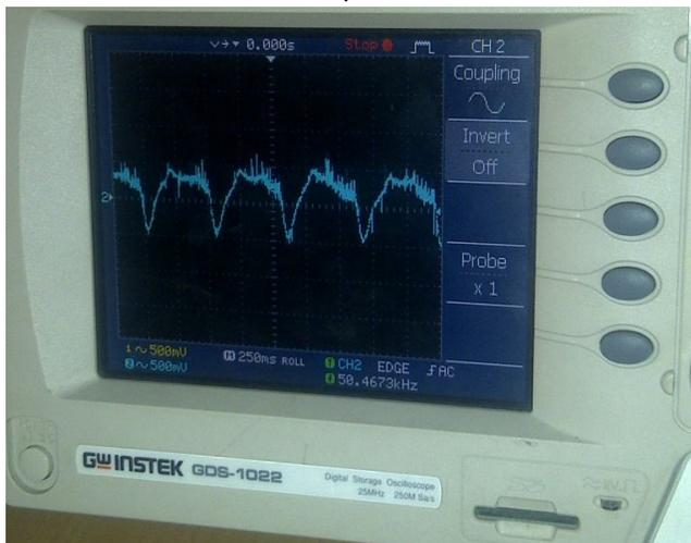
**Fig.10** Obtained Carotid artery PPG Signal at the neck
