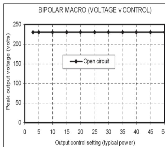
Fig. 8 Graph of Voltage vs. Control for Bipolar diathermy
