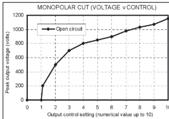
Fig. 6 Graph of Voltage vs. Control for Monopolar diathermy
