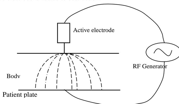
Fig.3 Basic principle behind the electrosurgical machine.
