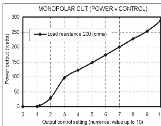
Fig. 5 Graph of Power vs. Control settings for Monopolar diathermy.
