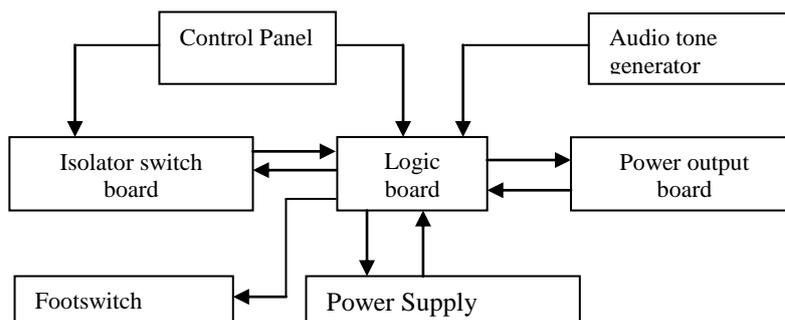
Fig.4 Block diagram for surgical diathermy machine.
