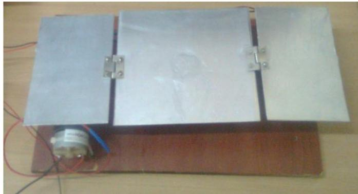
Fig.5 Proposed automated bed system with motors on each side for UP and DOWN conditions.
