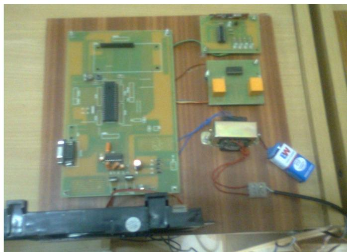
Fig.6 RF receiver section of the proposed system with PIC microcontrollers along with window like set up to show OPEN and CLOSE conditions.
