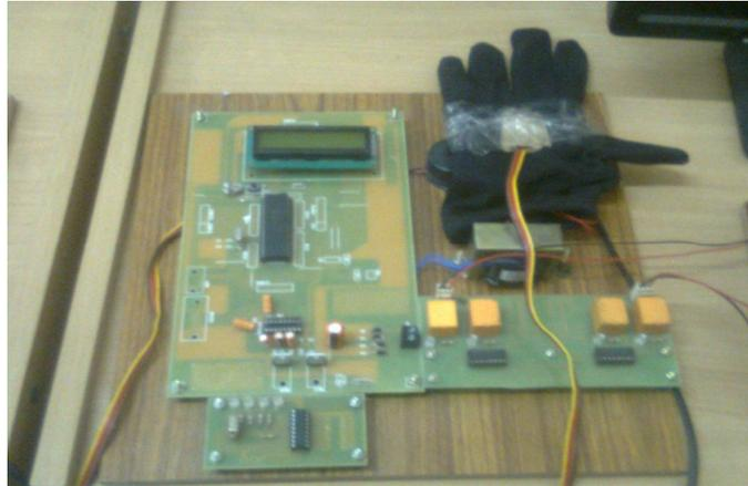
Fig.4 Transmitter section of proposed system with MEMS accelerometer, microcontroller and relay to control motors.
