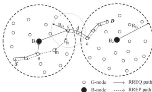
Fig 3. Processing RREP Packet
