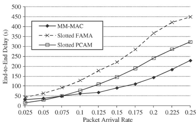
Fig. 4. Average delivery latency for the multiple-sink model.
