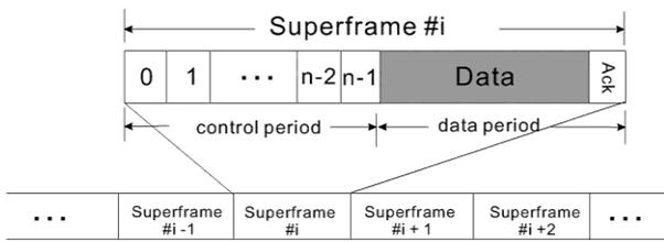
Fig. 2. Example of MM-MAC channel and slot allocation.
