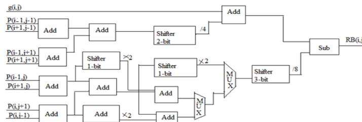
Fig 1.7.1. Architecture of the red and blue colors interpolator model 1 (RB\_M1 interpolator).
