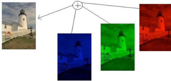
Fig 1.5 Construction of Color Image From Color Planes:
