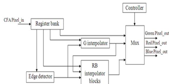
Fig 1.2 Block diagram of Proposed color Interpolation processor
