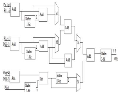
Fig 1.6.2. Architecture of the green color interpolator (G interpolator).
