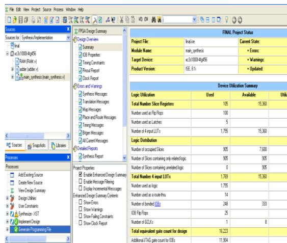
Fig 2. Total Equivalent gate count
