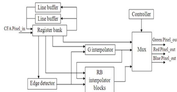
Fig 1.1 Block diagram of color interpolation processor.
