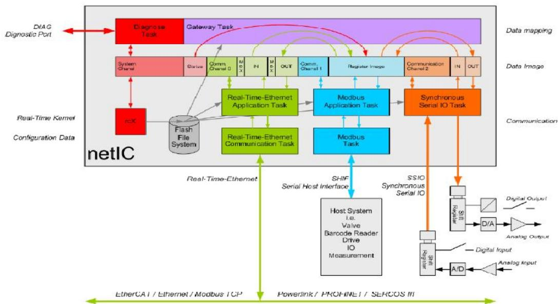
FIG.1 Data Transfer Process in Gateway
