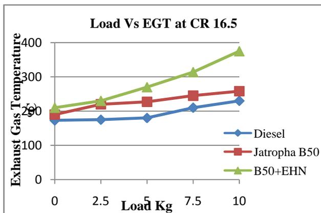
Fig. 4 Variation of exhaust gas temperatures with load of engine for different fuels
