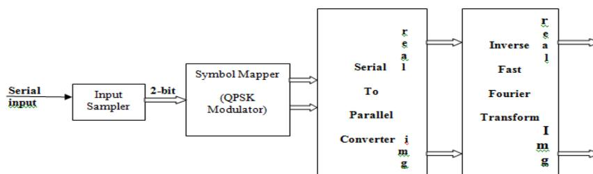
Fig. 1 OFDM transmitter
