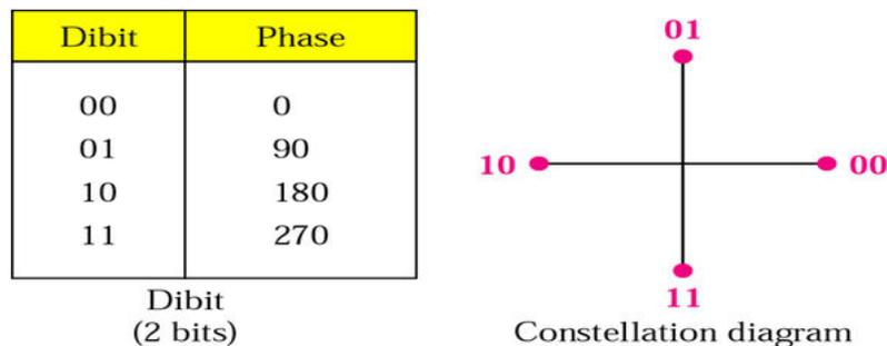
Fig. 3 Constellation diagram of QPSK modulation
