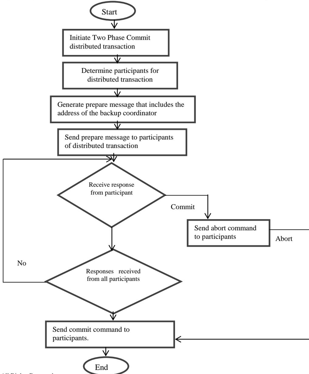
**Figure 1.1 Use of backup coordinator in a 2PC protocol flowchart**
