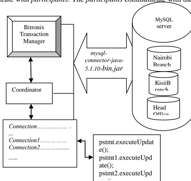
**Fig 1.3 Overall simulation architecture (Abuya et.al, 2015)**
