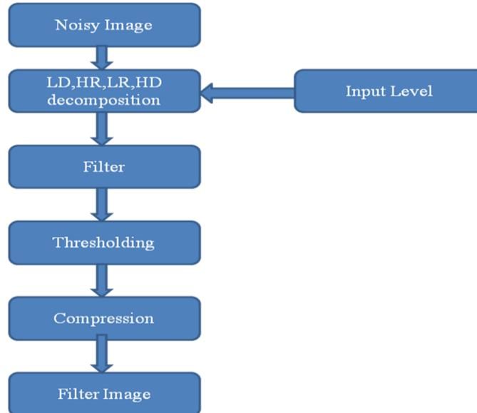
Fig. 2 Flow chart of the noise removal process
