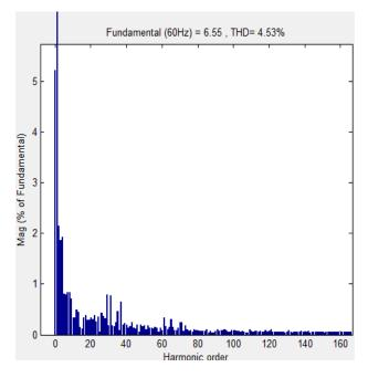
Fig.17. FFT analysis of source current
