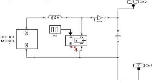
Fig.7. Boost Converter Circuit
