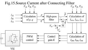
Fig. 16. Control diagram for the fully tuned branch.
