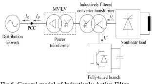
Fig.6. General model of Inductively Active Filter
