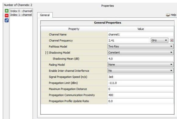
Figure 5: Channels configuration.
