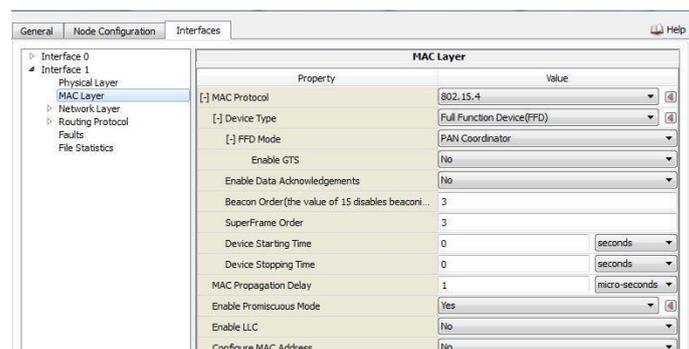
Figure 6: MAC configuration for MPDS on 802.15.4.
