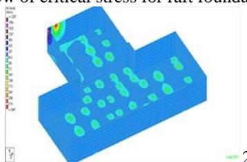
Figure 4 (c): STADD pro 3D modeled view of critical stress for raft foundation and retaining wall.
