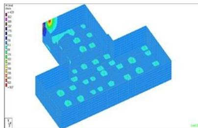
Figure 4 (a): STADD pro 3D modeled view of critical stress for raft foundation and retaining wall.
