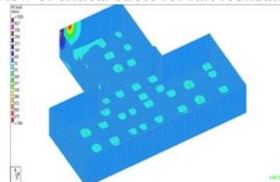
Figure 4 (b): STADD pro 3D modeled view of critical stress for raft foundation and retaining wall.
